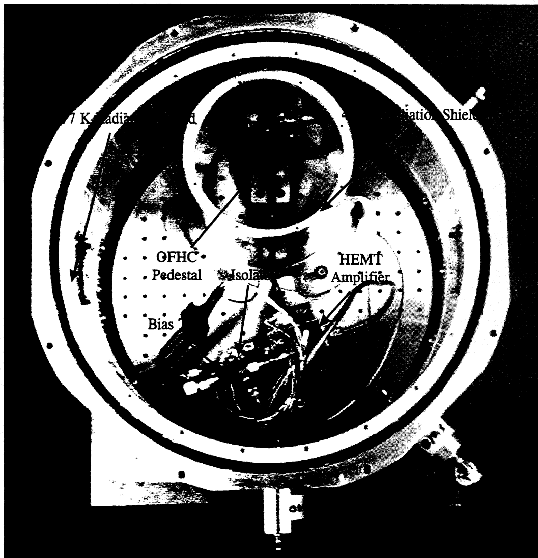
Figure 3: Top view of the IRLAB dewar showing the dc and IF connections.
