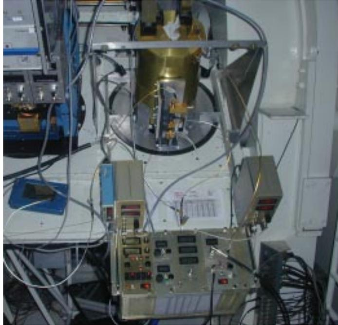
The receiver is a downward-looking cryostat at the top of the photo. The horn antenna is also mounted to the cryostat. The receiver is housed in a white cylindrical enclosure. The horn antenna is used to suppress radio frequency interference (RFI) as a part of the system.
