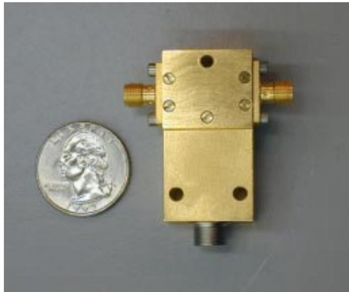
The assembled amplifier is shown in Figure 2. The length of the device is approximately 1.5 mm. The device is mounted on a substrate and has several pins for DC bias and RF connections.
