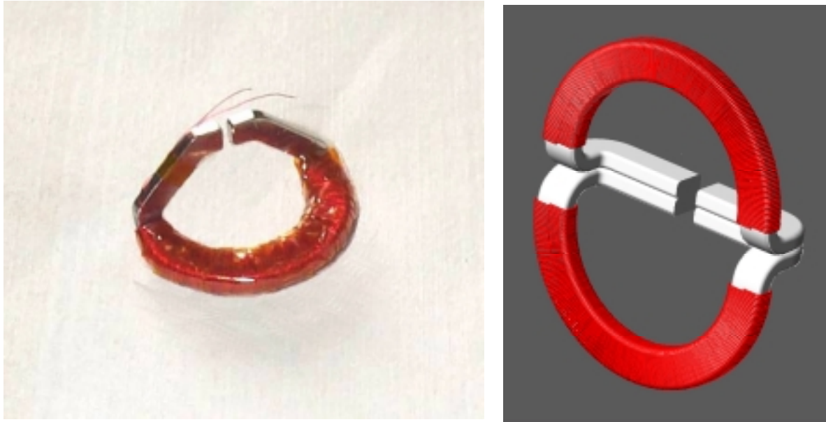
Figure 8. One half of the cryoperm electromagnet designed for Band 1 (1100 turns); artist's view.
