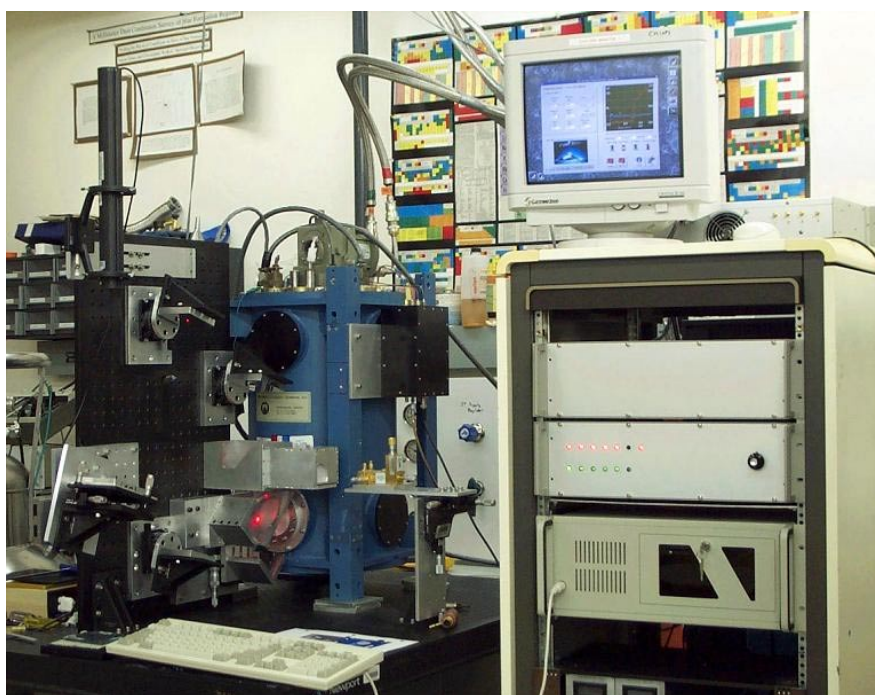
Figure 2: PoleStar frontend and control electronics during testing at SORAL.
