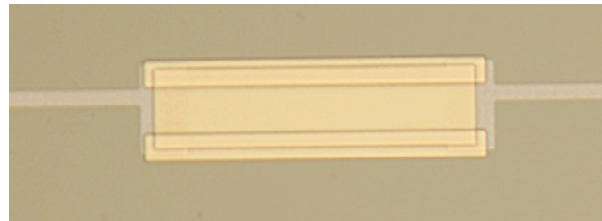
Figure 4. Photo of the Mo/Au TES with normal metal bars brighter at the edges along the direction of current flow. The length of the device is \sim 2 mm.
