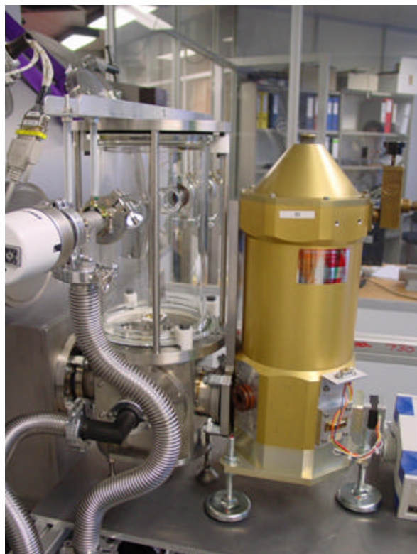
Fig.4: Picture of the gas cell (left) and of the hot/cold load source (golden cryostat) mounted onto the HIFI test setup.
