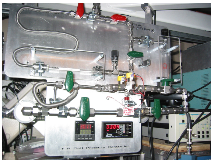
Figure 6. The manifold for creating a trickle flow of \text{CD}_3\text{OH} gas to the FIR laser tube.
