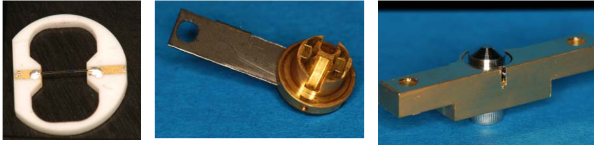
Figure 3 Left: Alumina device mounting ring with a SIS device mounted with two dots of silver epoxy. Middle: device mount with alignment spring attached. The heater is mounted in the backside of the device mount. Right: The pressure unit that pushes the device mount against the horn. The bullet-like part is pushed forward with an (internal) stack of spring washers.
