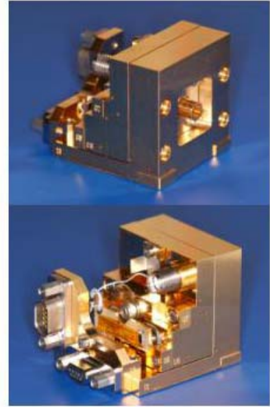
Figure 1 Left: Exploded view of the mixer block. Right: Front and backside view of an assembled mixer unit
