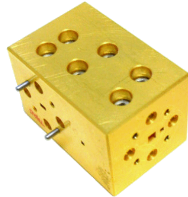
Fig. 5. Photograph of the WR-10 OMT.
