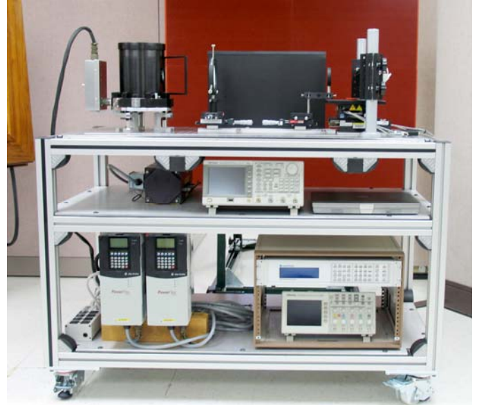
Fig. 4. Photograph of our terahertz imaging and spectroscopy system assembled on a mobile cart platform.
