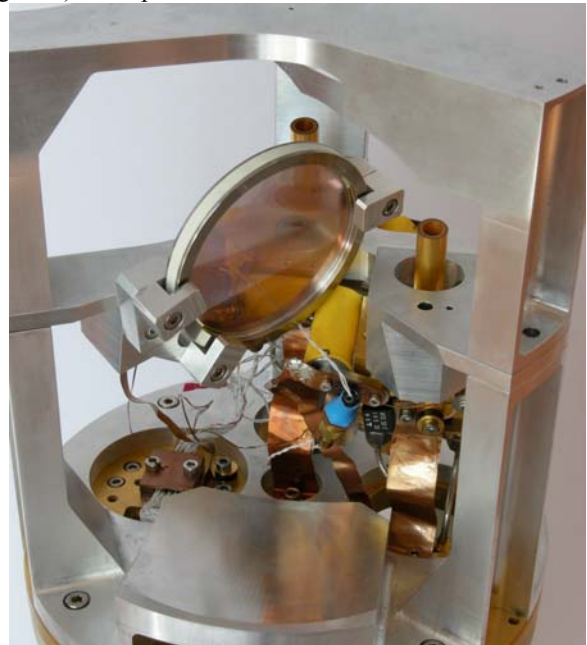
Figure 1. The Band 7 cold optics. Mirrors M1 and M1R are at the top, partly hidden; horns at the back, circular grid in middle, mirror M2R bottom foreground.
