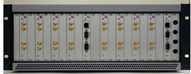
Figure 7: Measured Allan variance of the Supercam spectrometer system, including the Caltech IF processor. Allen time is 650s (top). The Supercam spectrometer system, built by Omnisys AB (bottom). This single 3U crate can process 16 GHz of IF bandwidth at 250 kHz spatial resolution. It consumes less than 200W of AC power.
