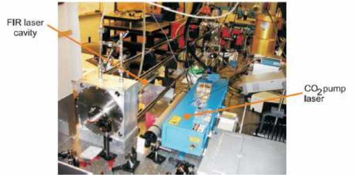
Figure 11. Photograph of the terahertz gas laser source.
