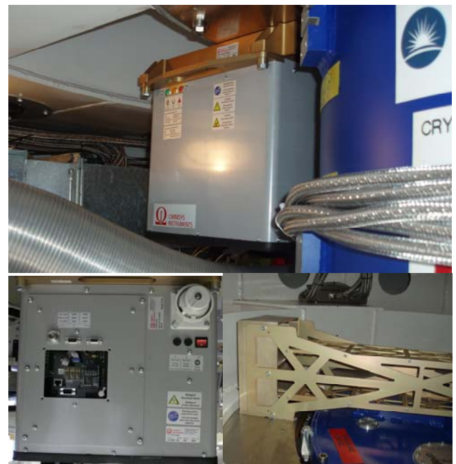
Fig 11. The radiometer installed on an ALMA antenna.
