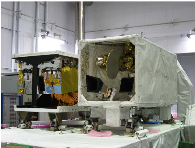
Fig. 2. SMILES (right) on the EF Pallet. The pallet was launched via H-II Transfer Vehicle (HTV) and carries to the EF. The left of SMILES is US HREP. The photo was taken in May 2009.
