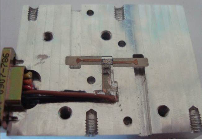
Fig. 5 Commercial chip packed in a split block.
