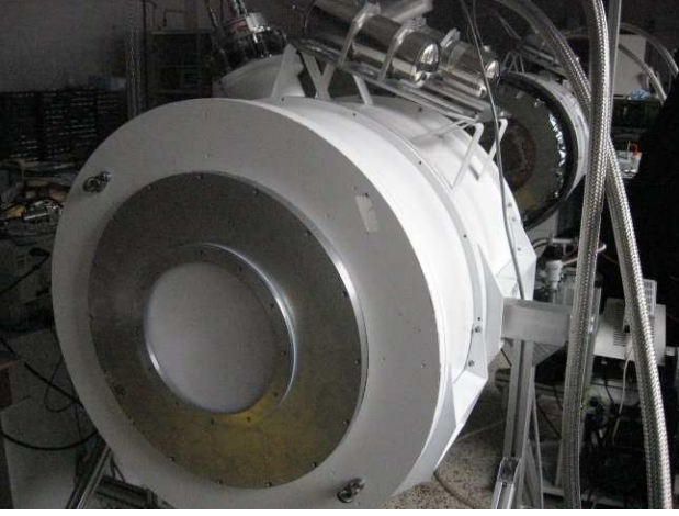
Fig. 2 CLOVER's LF cryostat.
