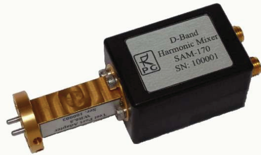
Fig. 6 A packaged harmonic mixer includes a replaceable waveguide test-port adaptor, an internal isolator and a LO/IF diplexer. IF and LO have separate SMA connectors.
