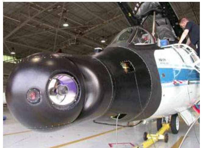
Figure 7: The WAVE system mounted on the nose of a WB-57F. ATOMMS will replace the optical telescope in this system. A microwave transparent radome will replace the front skin and optical window.
