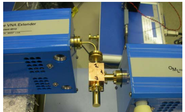
Fig. 12. Photo of the OMT during Pol 1 transmission measurement with the vector network analyser.
