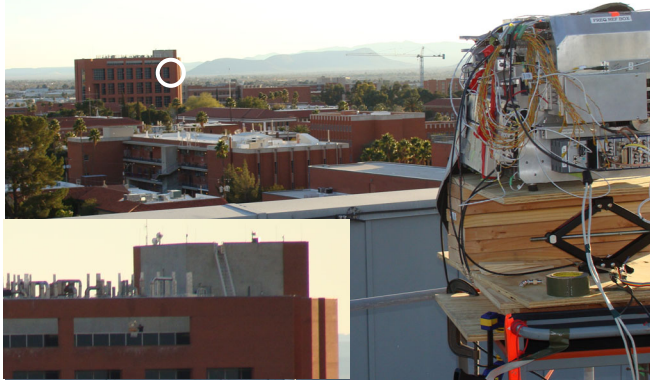
Figure 9: View of the Gould Simpson building from AME building. ATOMMS transmitter is shown in right side of the figure on the AME roof. The insert in the lower left shows the ATOMMS receiver on the 11th floor roof of Gould Simpson.
