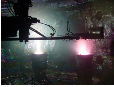
Fig. 5. Photograph of the bi-layer fabrication with niobium (left) and aluminium (right) sources by magnetron DC/RF sputtering under argon atmosphere.
