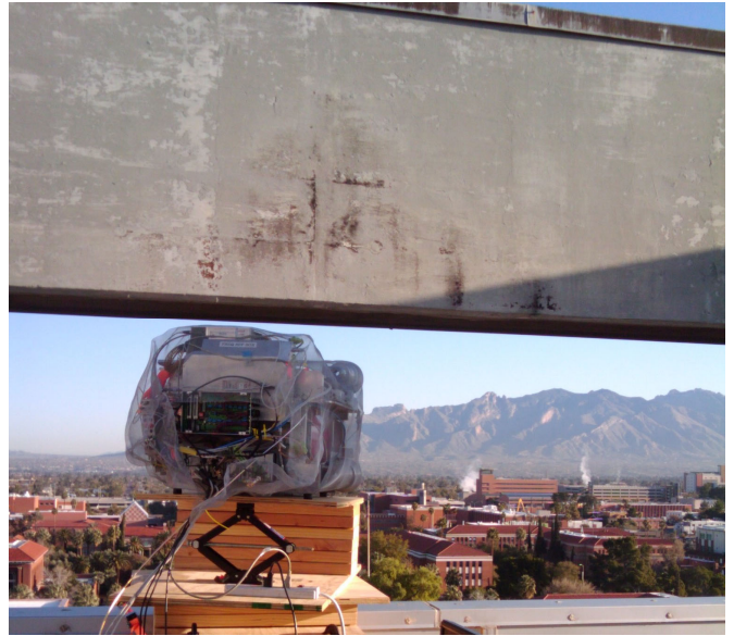
Figure 10: ATOMMS receiver on Gould-Simpson looking back at the transmitter on AME located in the white circle. Photograph taken on the morning of March 12, 2010. The cement beam above the ATOMMS receiver is in front of and above the ATOMMS receiver and is part of a façade that encircles the entire building.
