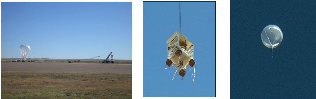
Figure 5: (Left) Balloon inflation is nearly complete at 9:50 AM on 15 October. (Center) STO launches at 10:03 AM, and reaches float altitude two hours later, hanging overhead (Right) for nearly the entire flight, and landing < 100 miles away at 1:15 AM on 16 October.
