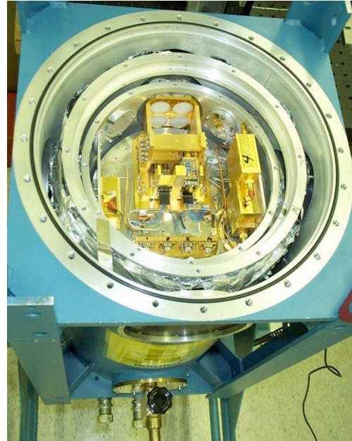
Fig. 2. The PoleStar 4-pixel heterodyne array for the 850 GHz band. The mechanical and electrical complexity of modular components limits pixel number.
