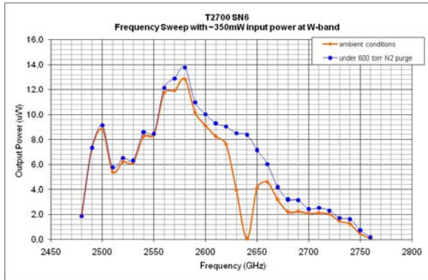
Figure 6: Performance of the LO chain at room temperature. Measured power under ambient conditions shows loss due to water absorption. In a nitrogen environment, a peak power of 14 microwatts at 2580 GHz has been measured. This is a record for a solid-state tunable room-temperature source at this frequency.
