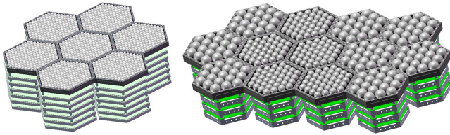
Fig. 11. CAD drawing of the proposed POLARBEAR-2 focal plane (left) and LiteBIRD focal plane (right). POLARBEAR-2 focal plane mounts seven hexagonal wafers with lumped diplexer with total of 7588 bolometers. LiteBIRD focal plane uses two types of detectors. There will be eight low frequency wafers with larger lenses and five high frequency wafers near the center of the focal plane. LiteBIRD focal plane will have 2022 bolometers total.
