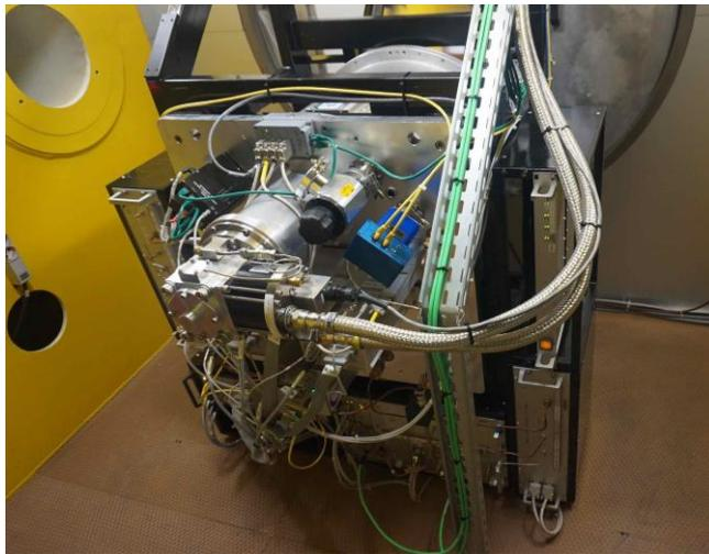
Fig. 1. Receiver installed in the 10<sup>th</sup> NOEMA 15m antenna. All critical electronics is directly mounted on the top plate.
