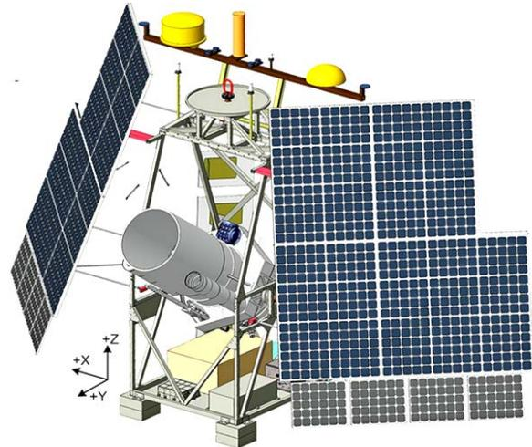
*GUSTO* ballooncraft and payload include a 0.9 m telescope, cryogenic THz receivers, and a gyro stabilized pointing system to provide an unparalleled galactic-extragalactic survey capability.
