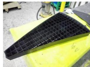
(b) CFRP tubes array core
