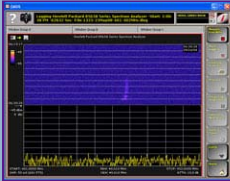
Figure B: A Low Earth Orbiter turns off its downlink in the middle of a pass over Green Bank in a test on 5/24/08 in preparation for the Phoenix Mars Landing on 5/25/08.
