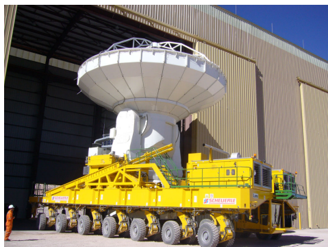
July 7: An ALMA transporter moves a VertexRSI antenna for the first time, transporting it from inside the assembly building to an outside pad.
