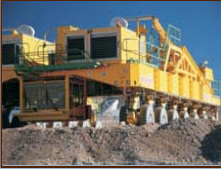
Figure 4. One of two massive ALMA transporters undergoes tests at the 16,500 foot Array Operations Site. The APEX antenna, which is similar to the Vertex prototype antenna, can be seen through the undercarriage. Photo by A. Beelen.
