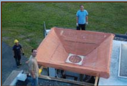
Figure 1: The phased array receiver and ground screen mounted in the Green Bank Indoor/Outdoor test facility. Clockwise from top are BYU students Jacob Waldron, Jonathan Landon, and Jiyoung Son.
