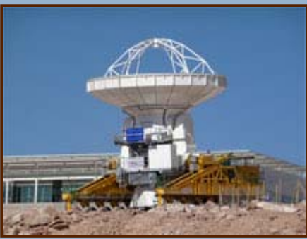
Figure 1. Antenna transporter Lore moves a Vertex antenna past the OSF Technical Buildings to a testing site.
