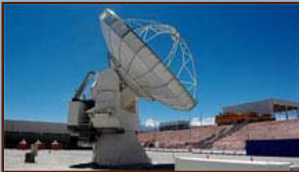
Figure 2: Now outfitted, a Vertex antenna undergoes tests at the OSF Technical Building. An antenna transporter can be seen near its shelter in the background. Further in the distance, the Licancabur Volcano stands sentry. Photo courtesy Denis Barkats.
