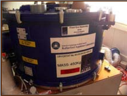
Figure 2 The third ALMA Front End was shipped intact from the European Front End Integration Center and arrived in fine shape. After passing its tests, it is ready for installation in the third ALMA antenna. Photo courtesy D. Barkats.
