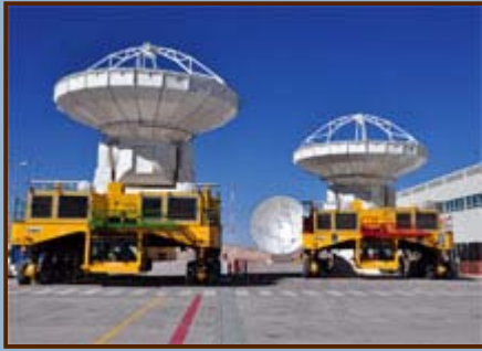
Figure 1. Two antennas constructed by Vertex ride on ALMA transporters at the Operations Support Facility (OSF) in Chile. An antenna constructed by Mitsubishi Electric Corporation (MELCO) is in the background. These three antennas have been conditionally accepted by ALMA and will participate in the first phase closure tests at the high-elevation Array Operations Site (AOS). © ALMA (ESO/NRAO/NAOJ)
