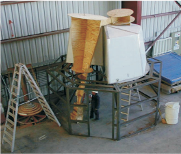
A mockup of the new Cassegrain focus feed structure and feed system were built and installed on a mockup of the receiver cabin as an aid in planning equipment layout in the receiver cabin.
