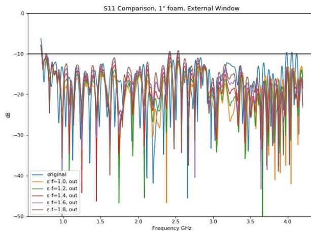
**Figure A1** compares the S11 results of all dielectric constants tested for the window in condition one, with results of the original model shown in blue. At higher values of dielectric constant, the S11 performance is worse than the original model. This emphasizes that the location of the window is a more significant factor than either the foam thickness or dielectric constant, and the window should be placed inside the feed's thermal gap, instead of the location in the original model.
