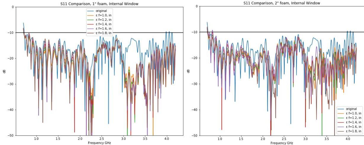
**Figure 4.** Figure 4a, at left, compares all dielectric constants tested in condition two, while Figure 4b, at right, compares all dielectric constants tested in condition three. Regardless of dielectric constant chosen, the performance of the window in each condition is notably improved from the original model (original results shown in blue). The window in condition two shows S11 results that are lower at the higher end of the band than those in condition three.
