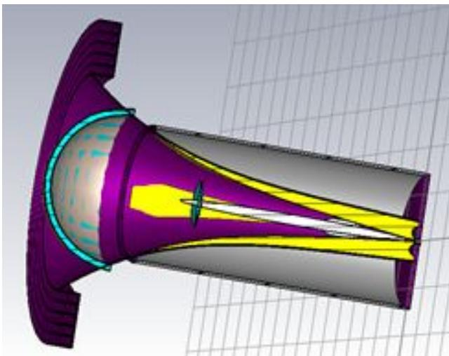
**Figure 1.** A cross sectional view of the feed horn as modeled in CST Microwave Studio. The full sized feed horn is approximately 1.5 meters long. The quartz window in question is the cyan and tan dome at the left of the model; all elements contained inside the window and grey can will be cryogenically cooled to 15 K, while external components will remain warm at ~290 K.
