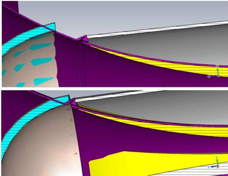
**Figure 2a.** The first condition under which the five dielectric constants were tested, with one inch thick support foam in the original window location shown in cyan, the inner quartz layer in tan, and the horn wall in purple.
