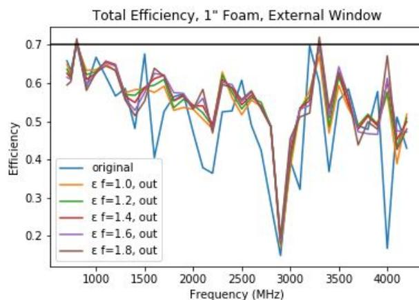
**Figure A2** compares the total efficiency results of all dielectric constants tested for the window in condition one, with the result of the original model shown in blue. Although the efficiency of the sandwich window shows an improvement over the original model, regardless of the dielectric constant, and even exceeds the 70% goal of the pulsar community, the S11 results from Figure A2 are unsatisfactory enough to invalidate these efficiency results.
