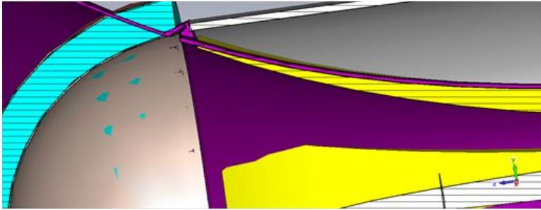
**Figure 2c.** The third condition under which the five dielectric constants were tested, with two inch thick support foam shown in cyan, where the entire window has been shifted into the thermal gap, in the same position as in Figure 2b.
