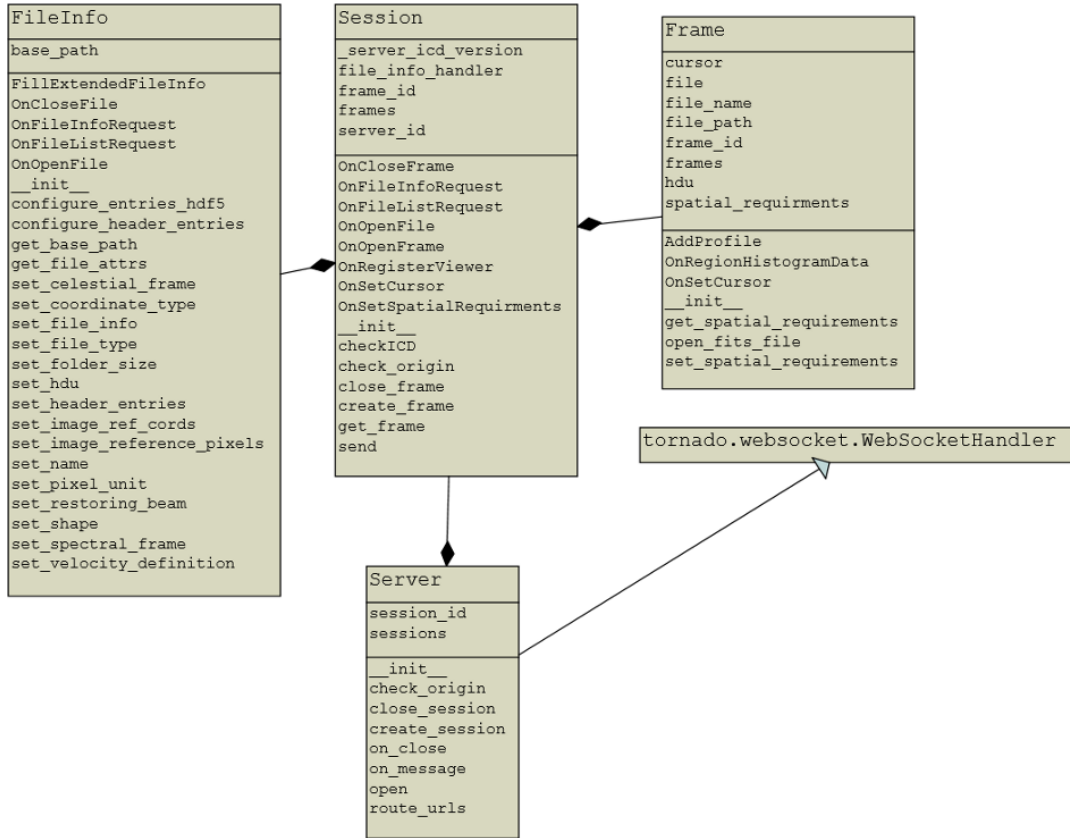
FIGURE 3. UML diagram for python back-end
